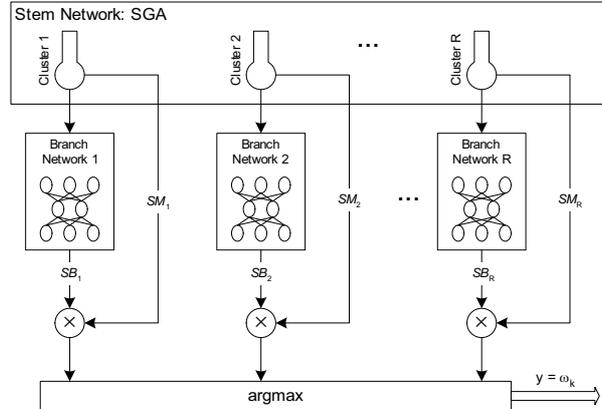
Fig. 1: CombNET-II structure
